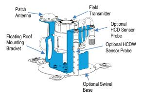
If the Swivel Base is not required, three strong magnets can secure the bracket onto flat steel surfaces. 3M VHB adhesive tape is used to secure the bracket if the surface is not steel (e.g. aluminium or composite floating roof).
