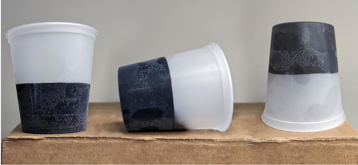
Figure 10: Crude oil viscosity increase demonstration at -25 °C.
